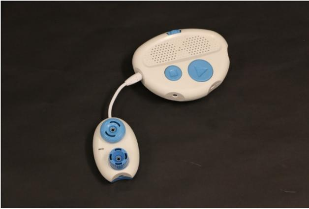
[Figure Caption:] A photo of a Play pod connected to the Code Jumper Hub at Port 1
