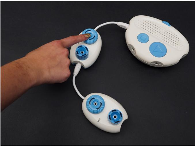
[Figure Caption:] This is a photo of the Code Jumper Hub and two Play pods. One Play pod is connected directly to the Hub at Port 1, and a second is connected to the opposite end of the first Play pod. A child's hand is pointing to the first Play pod, indicating tracing the code.
